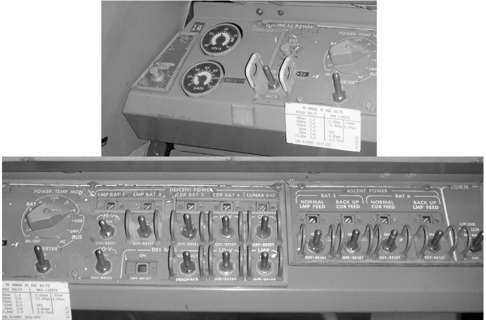
Figure 119: Electrical power system battery monitoring and selection
